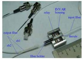
Fig. 3: Photo of the  $1 \times 2$  mechanical optical switch
