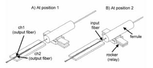
Fig. 2: Configuration of the switching mechanism
