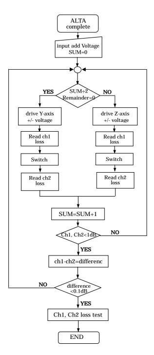
Fig. 7: Flow chart of ALTBA process
